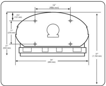
the unit is installed into the stud. Use toggles for holes on the opposite side.
